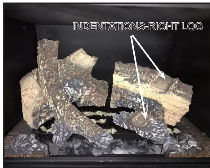
Figure 8. Location of Right Log Indentation
