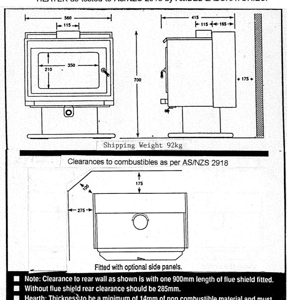
Hearth: Thickness to be a minimum of 14mm of non combustible material and must extend 300mm beyond firebox opening and 200mm to the sides.
