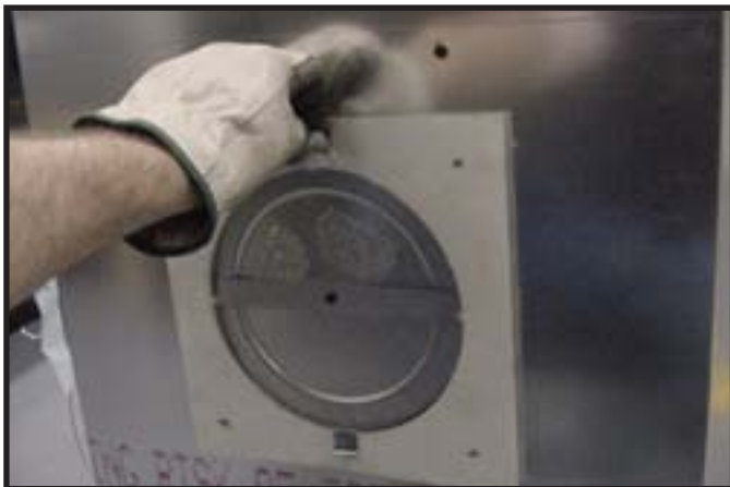
Figure 6.7 (Generic Appliance Shown) Fold the tabs toward the center of the seal cap (90°) and remove the insulation gasket.
