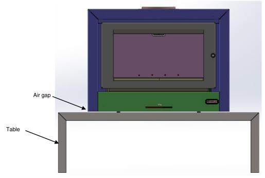
There must be an air gap between the bottom of the appliance and the top of a table. This is necessary to allow air flow to the appliance.
