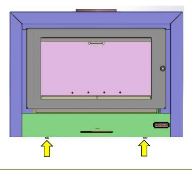
NOTE:- When installing this unit onto a table, make sure to leave the 4x bolts in place. The bolts are necessary to allow air flow to the underside of the firebox. The removal of these bolts will lead to overheating to the underside of the unit and eventually cause malfunction. The removal of these bolts could void your warranty.
