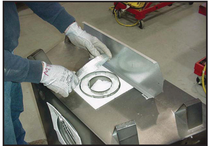
Figure 9.4 Remove the seal cap.
