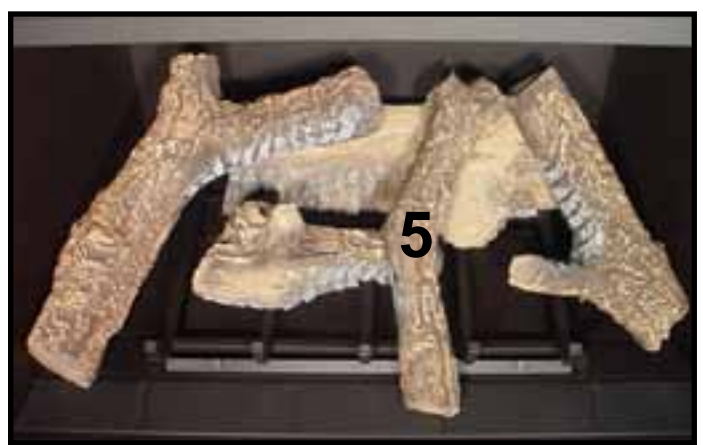
LOG #5 (SRV385-723): Position log #5 between the 3rd and 4th grate tines resting on the grooves in log #1 and log #2.
