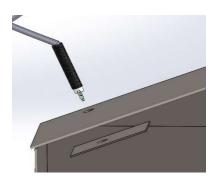
PUSH THE LIGHT FITTING THROUGH THE HOLE ON THE OUTER BOX AND INTO THE GAP BETWEEN THE PLATE AND OUTER BOX.
