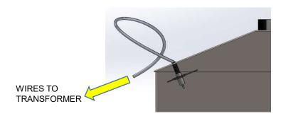
CONNECT 2x WHITE WIRES ON THE WIRING TO THE TRANSFORMER AND THE LIGHT WILL BE READY FOR USE
