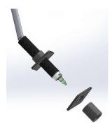
REMOVE ALL WASHERS AND NUT FROM THE WIRING. THEN ATTACH THE BULB TO THE LIGHT FITTING.
