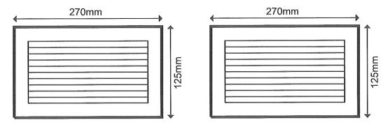
VENTILATION: An opening to outside with minimum free ventilation area of 400sq Centimetres for each decorative open gas fire
