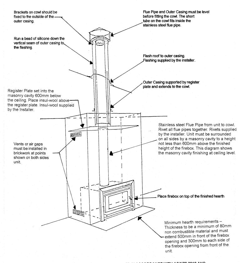
WARNING: THE APPLIANCE AND FLUE SHALL BE INSTALLED IN ACCORDANCE WITH AS/NZS 2918 AND THE APPRORIATE REQUIREMENTS OF THE LOCAL BUILDING REGULATORY AUTHORITY.
