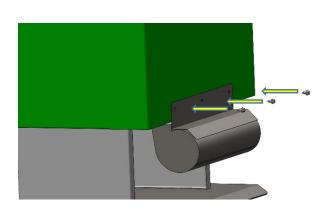
3. USE THE TEK SCREWS SUPPLIED AND FASTEN THE FAN ASSEMBLY TO THE APPLIANCE. A HEX HEAD SCREW DRIVE ON A DRILL IS REQUIRED.
