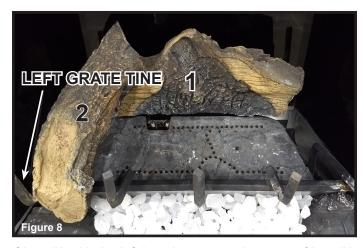
**Log #2 (SRV2164-702)**: Mate the slot located on the bottom of Log #2 with the left log placement tab on top of Log #1. After slot and tab have been fitted together, mate the groove located on the bottom of Log #2 with the horizontal grate bar and slide Log # 2 toward the left until it rests against the far left grate tine.
