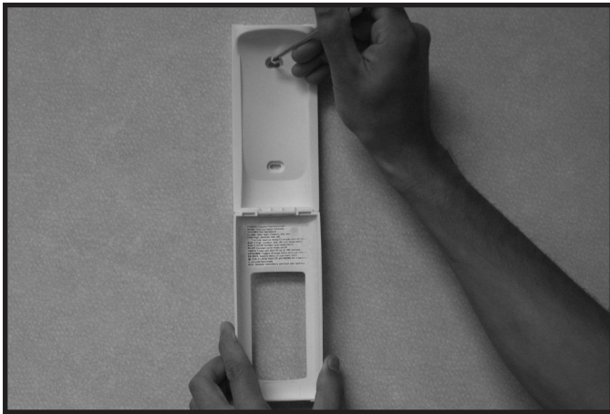
Figure 3.11 Mounting Remote Control Housing
