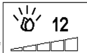
6b.9 Press the '+' and '-' button to select the 5 brightness of fuel bed and OFF settings.
