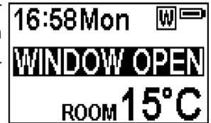
6b.36 After the indoor temperature has risen or a manual override of the warning (by operating remote control) has been done, the fire will return to normal working state.
