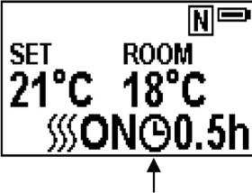
The heater can be automatically run by using daily timer and weekly timer on the remote.
