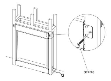
5.7a3 Position the appliance into the framework and secure it using fold out the brackets on the top and lower edge of this appliance.
