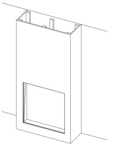
5.7a4 Cover the framework by panels or plaster board, it can be used directly against the sides and front of the appliance.
