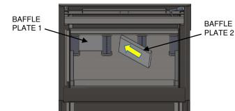
3. REPEAT STEP 2 PROCESS BUT THIS TIME MAKE SURE THE BAFFLE PLATE 2 SLIDES OVER BAFFLE PLATE 1.
